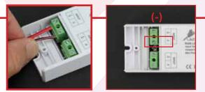
On the right side of the receiver, connect the LED ixture, being careful to match the correct color wires with the matching ports. Connect the positive wire and three other negative red, green and blue wires as noted on the wiring diagram on page 4. **Please Note: Do not exceed the Max Wattage ratings: 360W@24V DC, 180W@12V DC**
