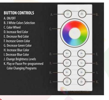
Press the ON/OFF button to turn the lights on or off.
